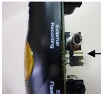
Jumper position in a "with battery" mode
