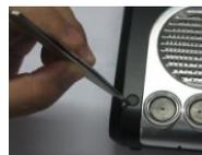
In such case, please remove the plug from the electricity power, open the 4 screw covers, remove the screws and open the front cover. Then connect the backup battery pack's connector to the PCB board where written BAT1.
